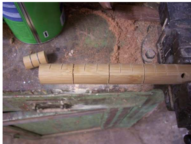
Dowel marked for cut-off and grooves for wire ribs. Each batch of 4 drums fits on a standard Pallet.
