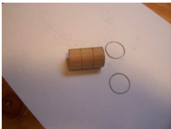
12mm diameter wood dowel cut to 30mm lengths, grooves cut to accept 0.9mm wire rings.
