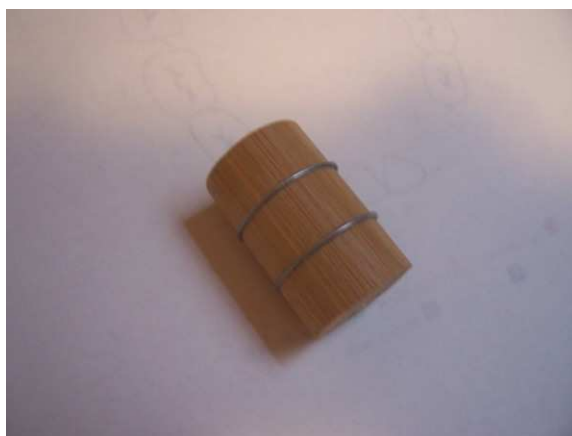
12mm diameter wood dowel cut to 30mm lengths, grooves cut to accept 0.9mm wire rings.
