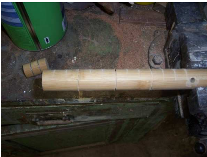
Dowel marked for cut-off and grooves for wire ribs. Each batch of 4 drums fits on a standard Pallet.
